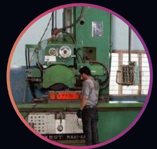
Special grinding machines can re-sharpen tools up to 3000mm X 1000mm
